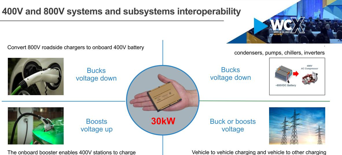
The onboard booster enables 400V stations to charge 800V vehicles
