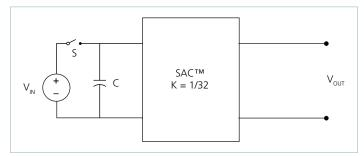
Figure 3 — Sine Amplitude Converter™ with input capacitor
