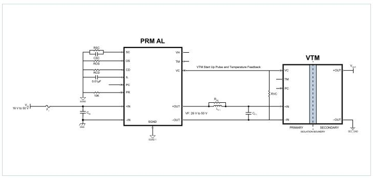
Using the MIL-COTs PRM<sup>TM</sup>, the output of the VTM is regulated over the load current range with only a single interconnect between the PRM and VTM and without the need for isolation in the feedback path.
